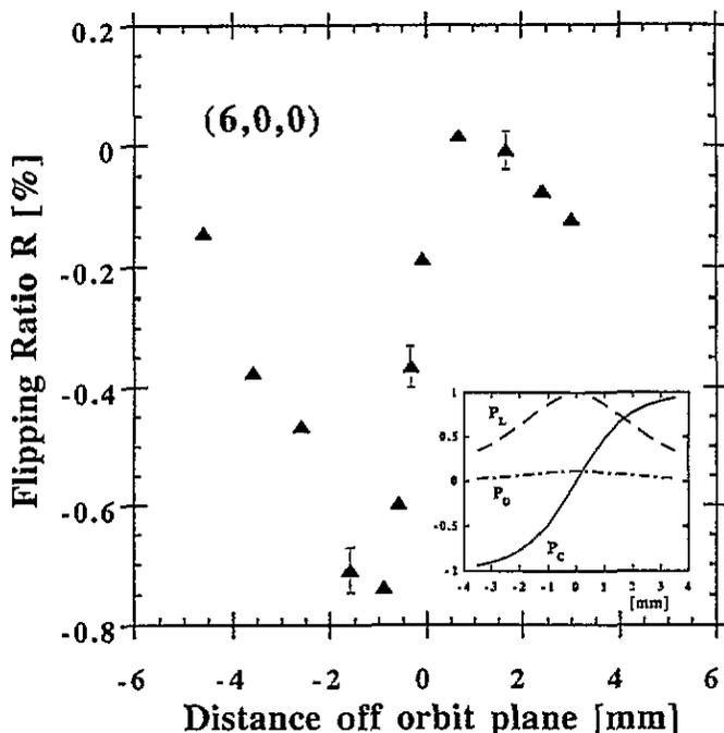
Figure 2. Observed flipping ratio  $R = (I^+ - I^-)/(I^+ + I^-)$  for the (6, 0, 0) reflection as a function of distance in mm off the synchrotron orbit plane. The data were measured at a distance of 33 m from the bending magnet source, using a 0.1 mm vertical slit. Inset: The calculated degrees of polarization (linear  $P_L$ , circular  $P_C$  and unpolarized  $P_U$ ) as a function of distance of orbit in mm.
