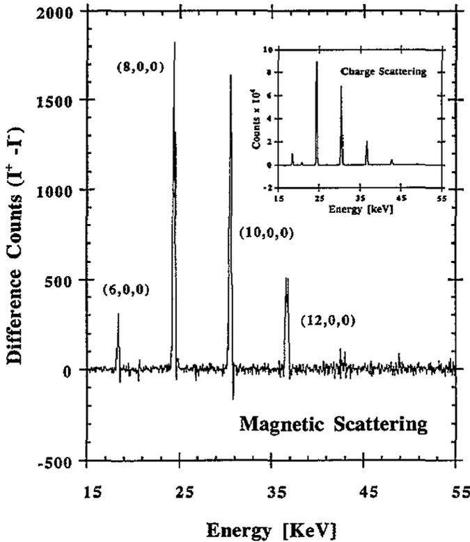
**Figure 1.** Typical magnetic difference profile obtained for  $(h, 0, 0)$  reflections of iron as a function of energy. Data were collected using the ID15 high energy asymmetric wiggler, with a 3 mm aluminium absorber placed within the incident beam to attenuate low-energy reflections. Inset: corresponding charge diffraction spectrum, measured with 10 minutes counting time.
